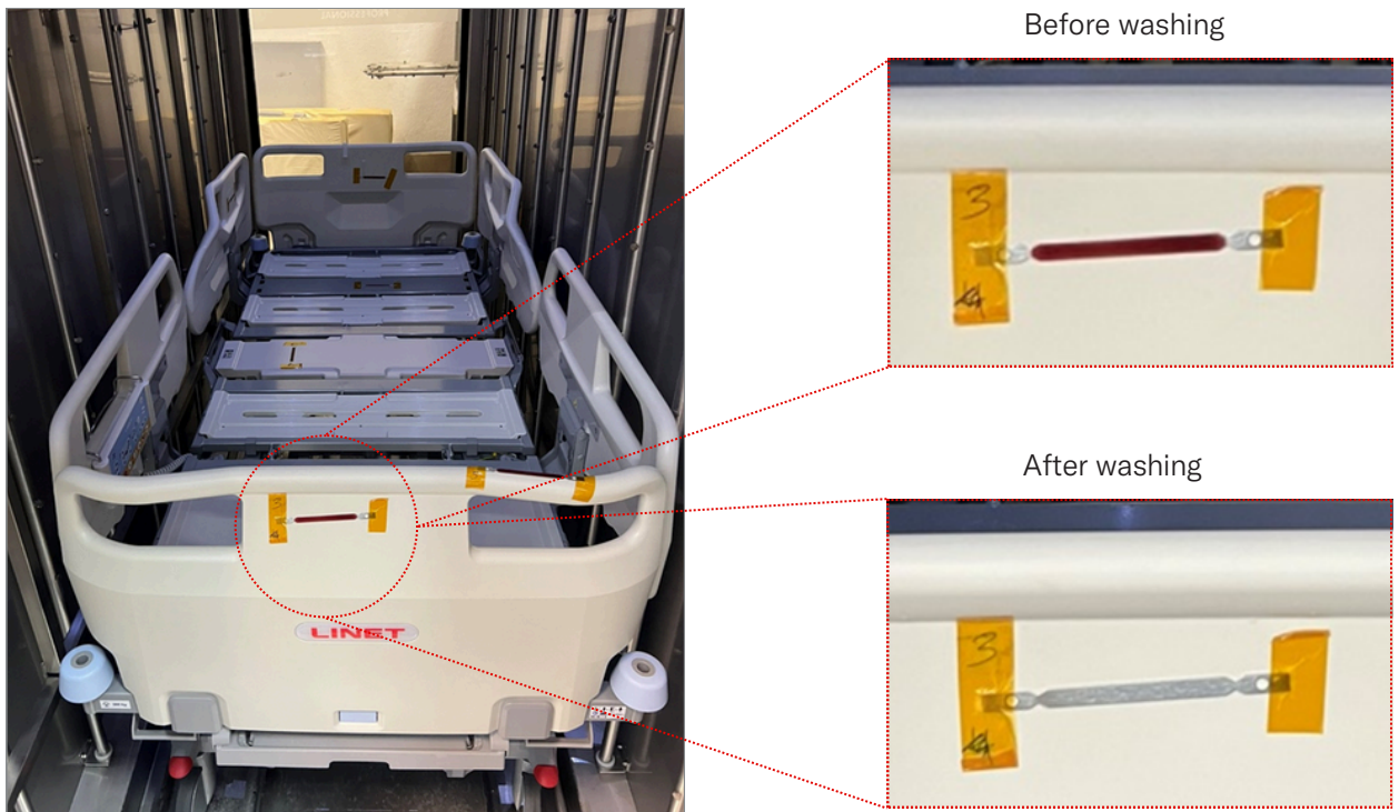
Image 5: Validation of biological testing by stripes, where is visible effect of cleaning process (after washing stripes are tested in laboratory)
