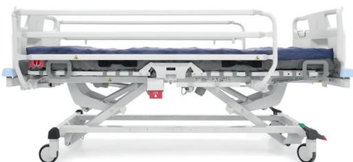
Single collapsible siderails cover three-quarters of the bed, ensuring a safe route for the patient to exit the bed in any situation. The simple design enables caregivers to easily lift or drop down the entire siderail with a single movement. By using single collapsible siderails, the bed can be configured to achieve a low height of 255 mm also.
