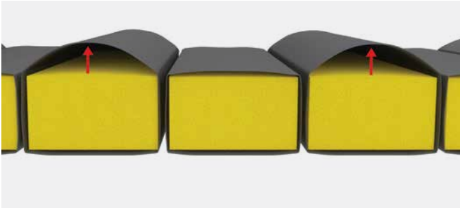
Active system with 2-cell alternation provides periodic pressure reduction.
