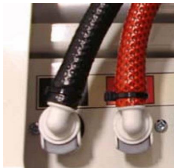
Fig. 7a Colour-coded Air Pipes (Symbioso 100)
