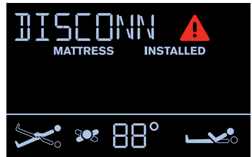
Fig. DISCONNECTED AIR PIPES
