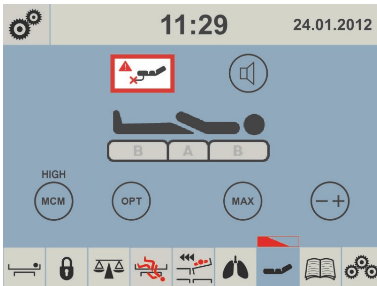
Fig. Alert – Disconnected Air Pipes
