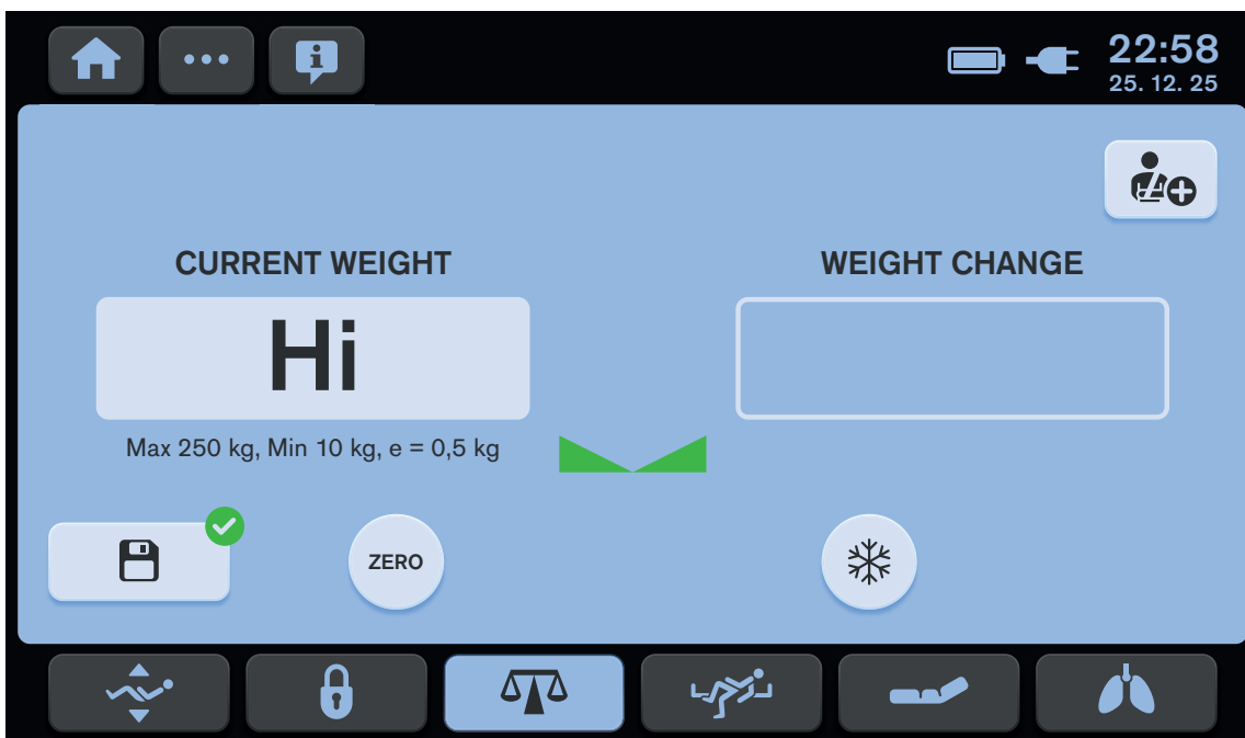
Fig. First degree of the bed overload (displayed Hi)
