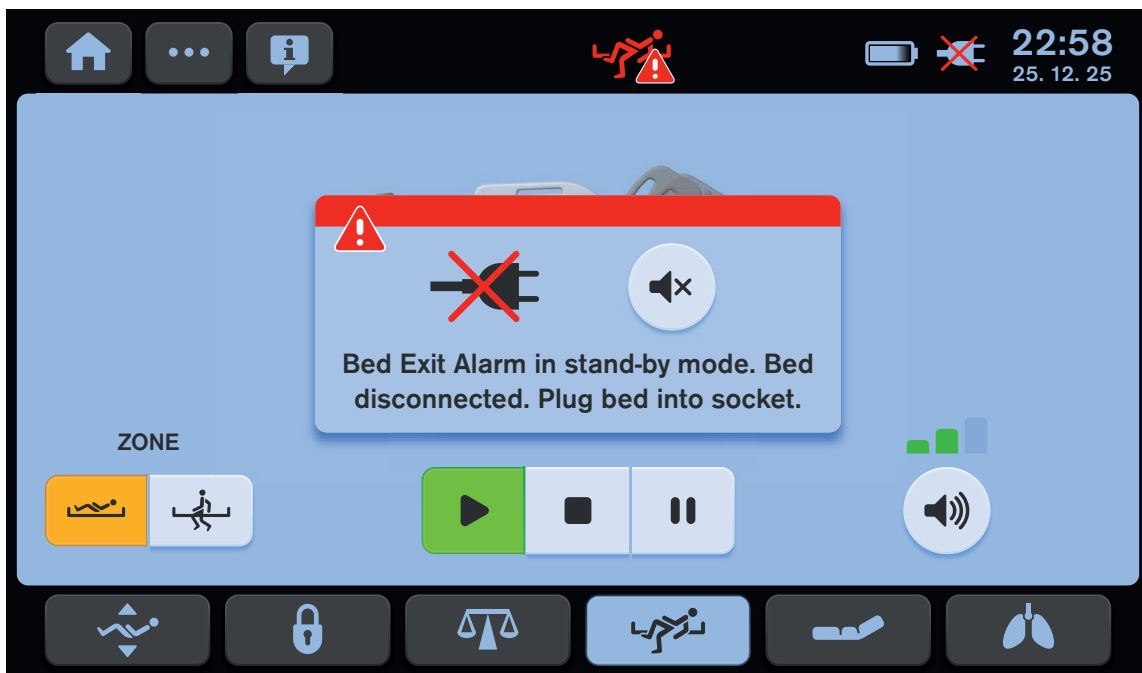
Fig. Bed Exit Alarm Monitoring is deactivated because of the bed disconnected from the mains power
