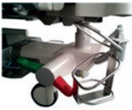
Fig. Oxygen Bottle Holder B – incorrect fitment
