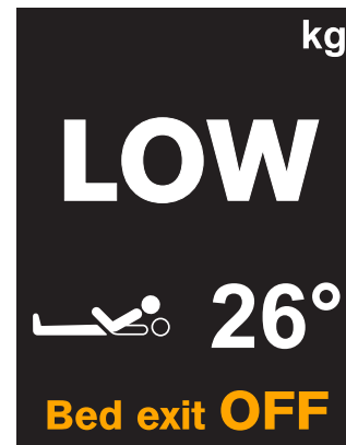
Fig. Charge insuffisante du lit (iBoard Basic)
