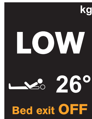
Fig. Charge insuffisante du lit (iBoard Basic)
