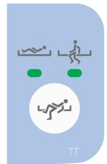
*Fig. Bed Exit Alarm Monitoring Button with 2 Green Indicators above*
