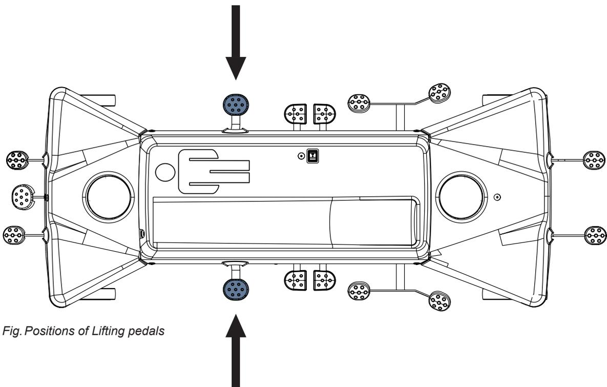
*Fig. Positions of Lifting pedals*
