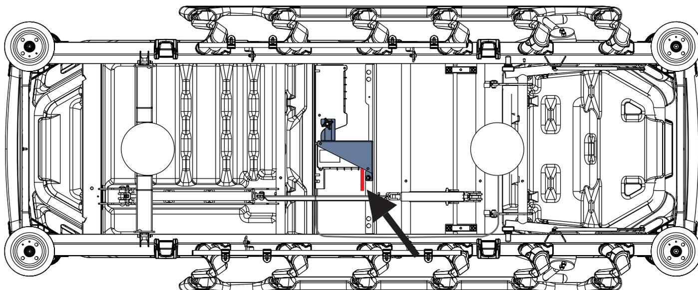
Fig. Battery Box with Battery Isolating Foil under the Seat Section (bottom view)
