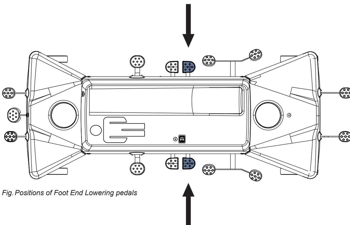
*Fig. Positions of Foot End Lowering pedals*
