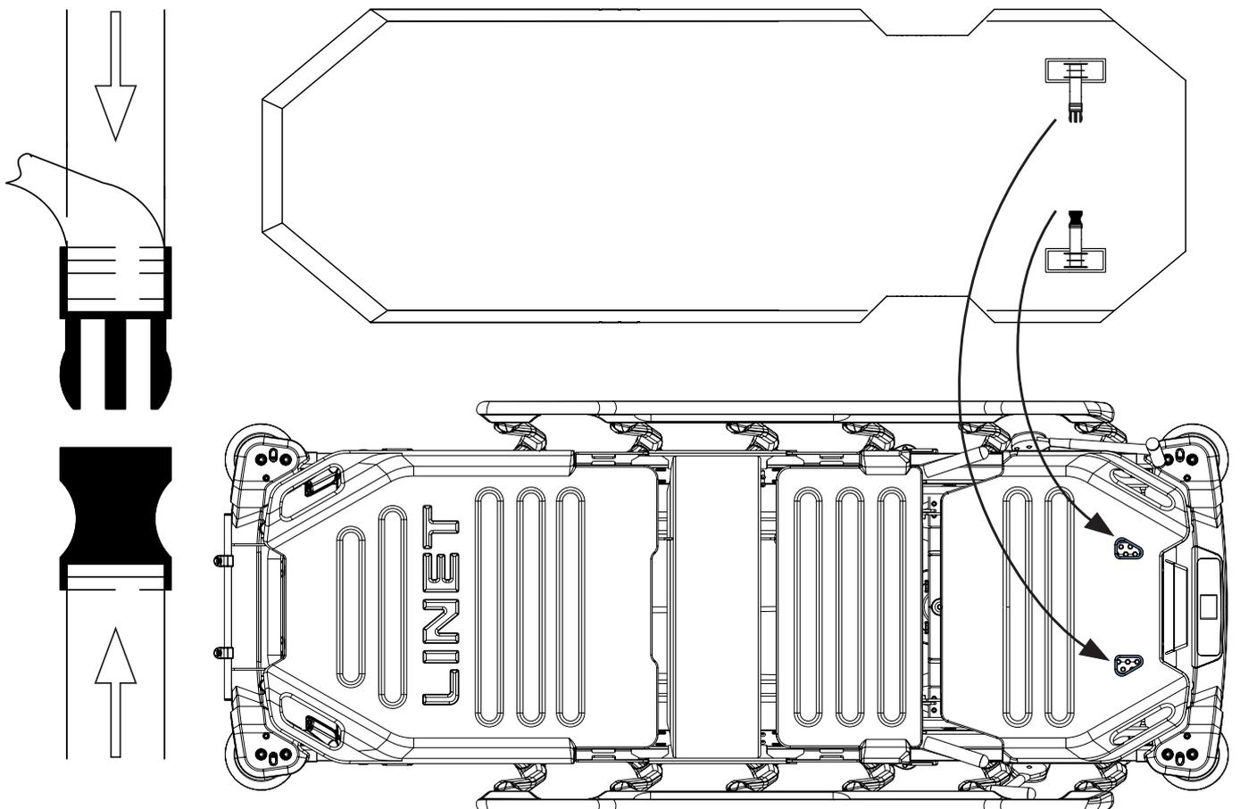
Fig. Fixation of mattress with straps on the Sprint 200 with 4-part mattress support platform
