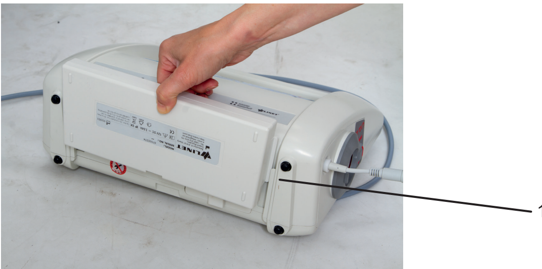
Fig. Fitting the accumulator pack
