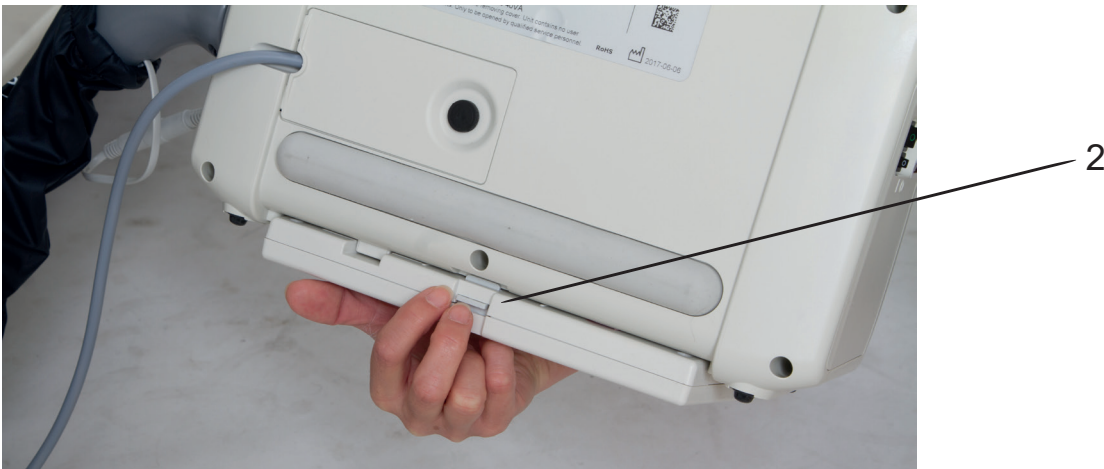
Fig. Removing the accumulator pack
