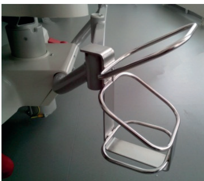
Fig. Oxygen Bottle Holder B – correct fitment
