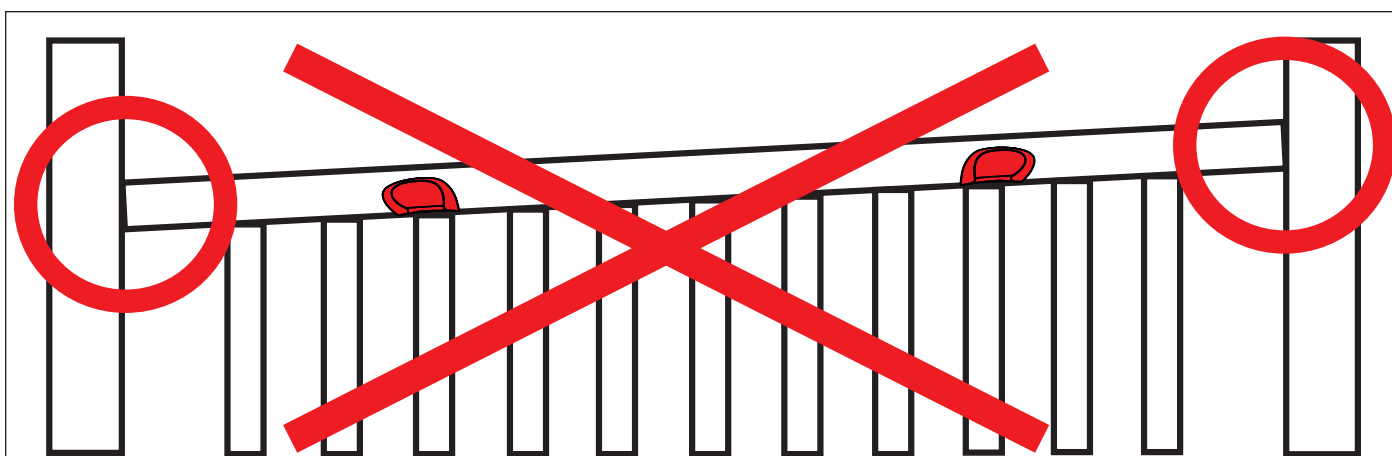
Fig. Incorrectly locked siderail
